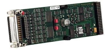
The mezzanine card M33 is a highly flexible M-Module for analog output signals. The isolated supply voltages can be generated by an on-board DC/DC converter. The output voltage range can be set to 0..10V, -5..+5V or -10..+10V for each channel by software. In addition, the current outputs can be used with 0..20mA or 4..20mA. The output load is driven to ground.
