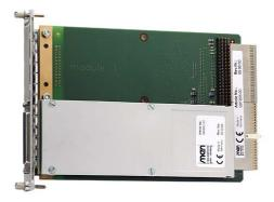
The F205 is a 3U M-Module carrier board for universal I/O on the CompactPCI® bus. It allows high flexibility in applications such as data acquisition or process control. The F205 is slightly higher than standard 3U format, providing enough space for two M-Modules while staying compatible with CompactPCI® housings
