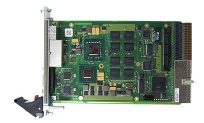
The F19P versatile 4HP/3U single-board computer is a continuation of MEN's proven range of Intel® CPU boards. It is equipped with the Intel® Core™ 2 Duo processor SP9300 running at 2.26 GHz and offering multi-core processor architecture from Intel® with full 64-bit support. The CPU card delivers an excellent graphics performance and is designed especially for embedded systems which require high computing performance with low power consumption.
